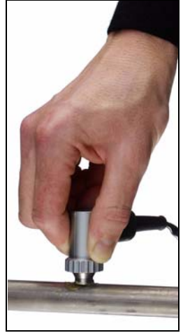
Wall thickness measurement
