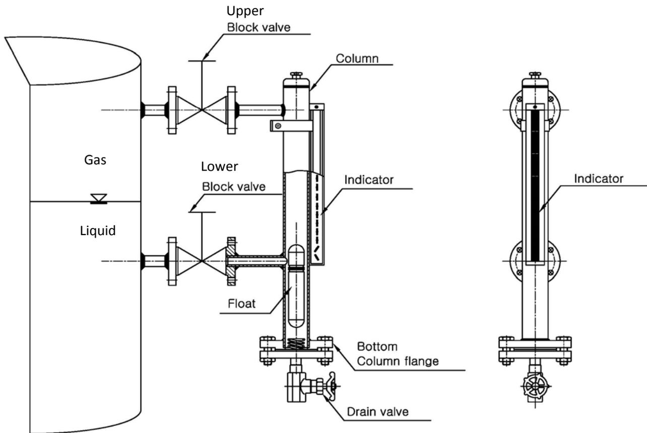
3) In case the indicator doesn't indicate a level after the inflow of fluid, check the following.
